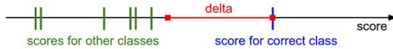
Figure 3.3: Visualizing the SVM loss margin. Class scores that fall within the red delta region contribute to the loss. Class scores that fall below the delta contribute zero loss. During training, the loss is minimized so that the correct class score is marginally higher than all other class scores [12].
